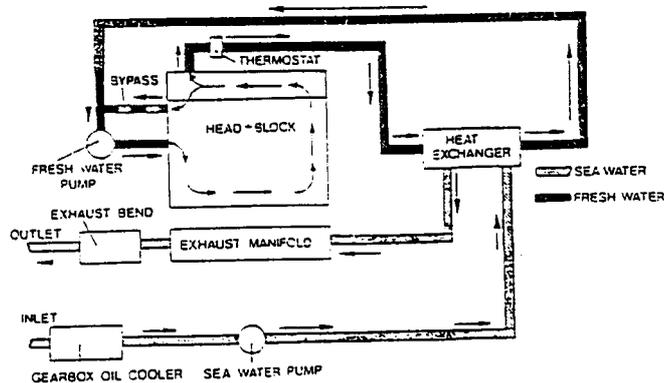
Heat Exchanger Cooling Layout - KD26/36
